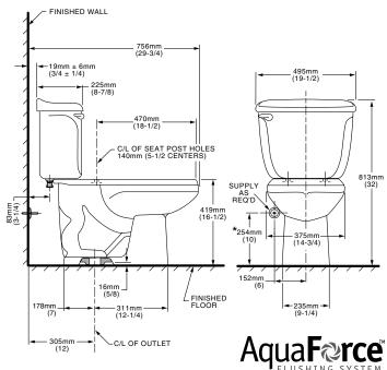
THIS TOILET IS DESIGNED TO ROUGH-IN AT A MINIMUM DIMENSION OF 305MM (12") FROM FINISHED WALL TO C/L OF OUTLET. SUPPLY NOT INCLUDED WITH FIXTURE AND MUST BE ORDERED SEPARATELY
